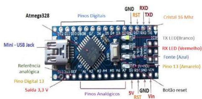
FIGURA 2. Plataforma Arduino Nano. (Adaptada - THE ENGINEERING PROJECTS)
