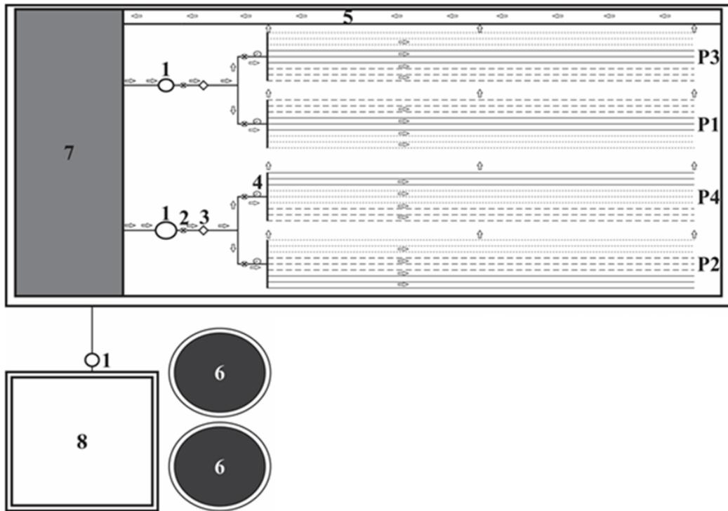
\*1 - Motor pump, 2 - Valve, 3 - Screen filter, 4 - Manometer, 5 - Channel, 6 - Reservoir for sanitary landfill leachate, 7 - Tank for the diluted effluent, 8 - Reservoir for public water, P1 - Drip unit operating with 70 kPa, P2 - Drip unit operating with 140 kPa, P3 - Drip unit operating with 210 kPa, P4 - Drip unit operating with 280 kPa, --- Dripper G1 (1.6 L h<sup>-1</sup>), — Dripper G2 (2.0 L h<sup>-1</sup>) and - - - Dripper G3 (4.0 L h<sup>-1</sup>).
