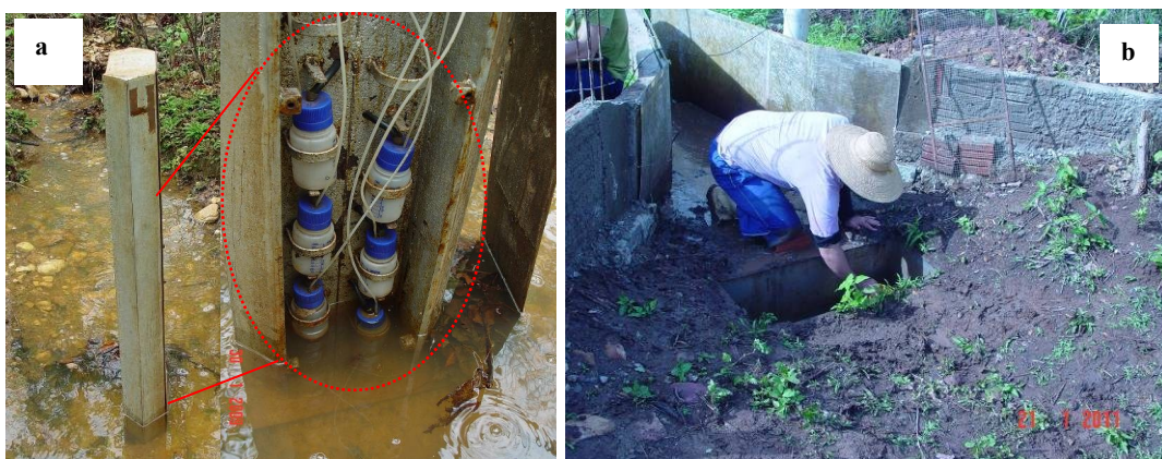
Figure 2. The tower to collect suspended sediments (a) and pit to collect dragged sediments in the watershed bed (b).
