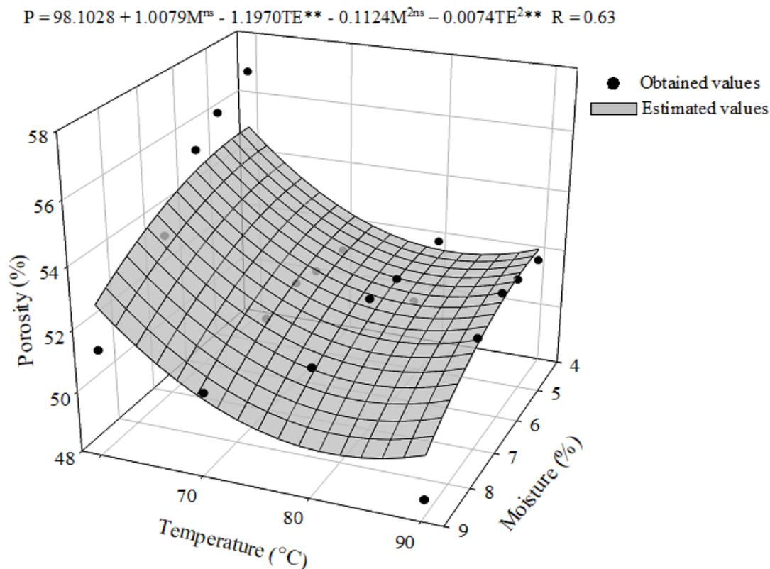
**Figure 6.** Total porosity (%) of macauba fruit kernels as a function of moisture and temperature. \*\* Significant at 1% and <sup>ns</sup> Not significant by the t-test.
