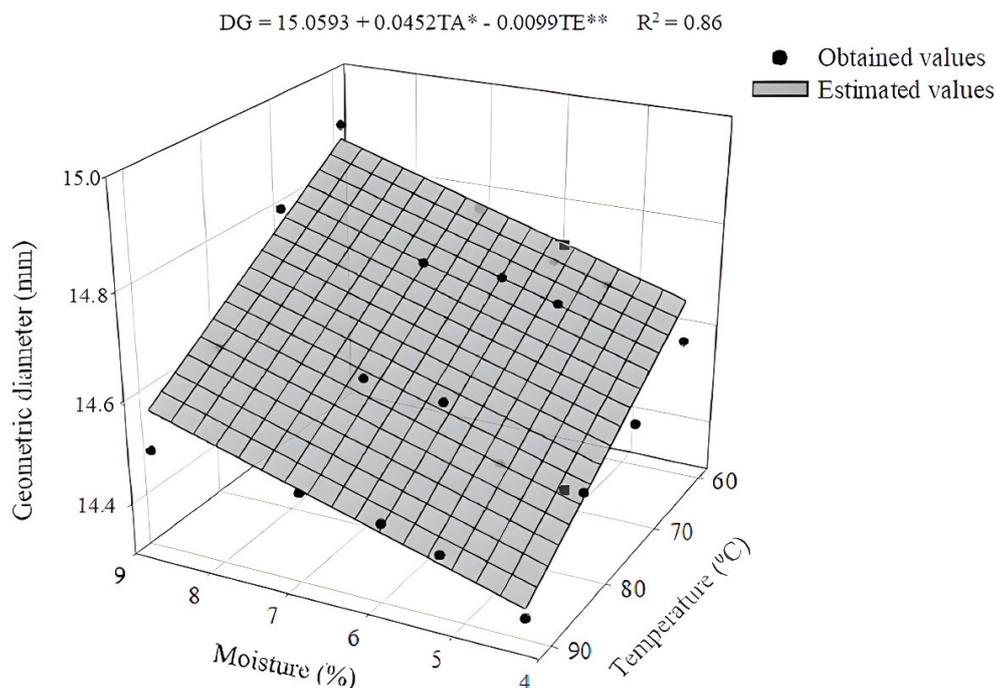
**Figure 1.** Geometric diameter (mm) of macauba fruit kernels as a function of moisture and temperature. \* Significant at 5% and \*\* Significant at 1% by the t-test.
