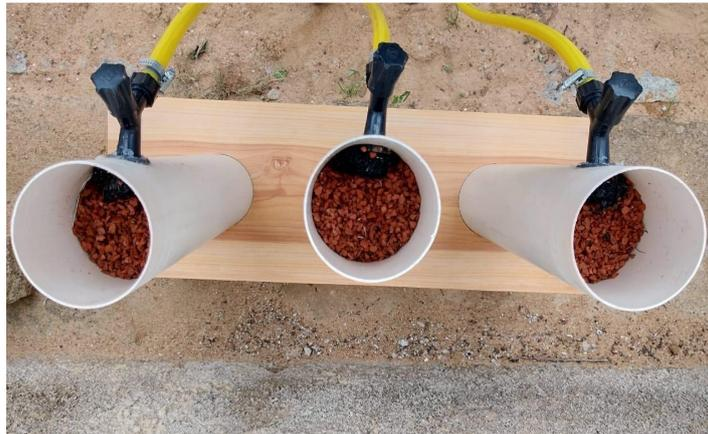
**Figure 2.** Filters filled with waste from the ceramic industry.
