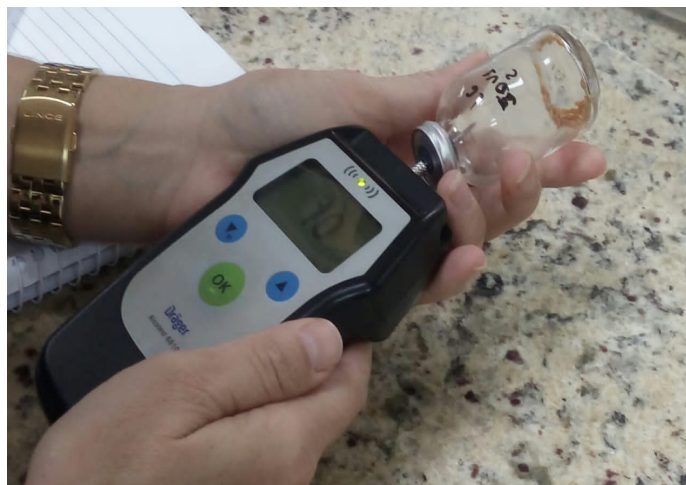
Figure 1. Equipment for assessing seed vigor based on ethanol production (breathalyzer).
