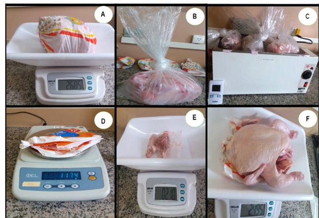
Figure 1. Steps taken during the Dripping test analyzes. (A) Weighing of the frozen carcass, (B) Carcass in a plastic bag, (C) Immersion in a water bath at 42^{\circ}\text{C} , (D) Weighing of the original packaging, (E) Weighing of the viscera and (F) Weighing of the carcass with offal and original packaging after thawing at 42^{\circ}\text{C} .
