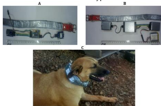
Figure 4: A. Placement of the modules on the collars. B. Modules in the cabinets. C. Prototype fixed to the collar
